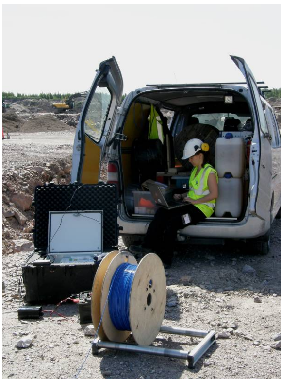
Figure 3: Distributed temperature system (DTS) measurements with fibre optic cable. Photo by I. Martinkauppi
