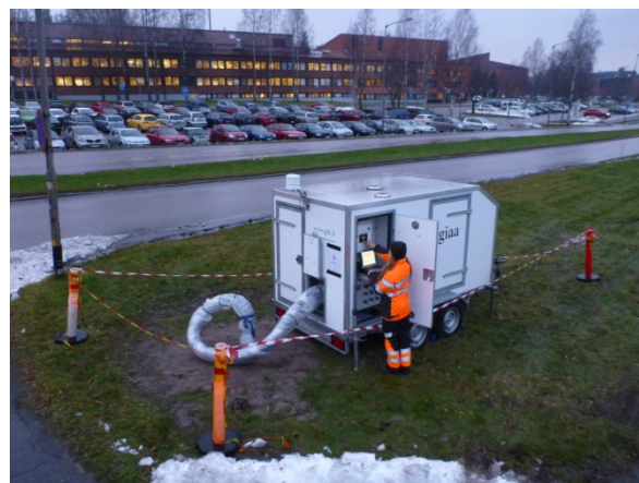
Figure 4: The Finnish thermal response test unit (TRT) in operation at urban building area. Photo I. Martinkauppi
